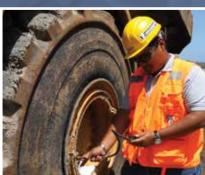
A high level of skill is required to carry out a quality earthmover tyre repair that can help you optimise the life of your Michelin tyres and therefore help reduce costs.
